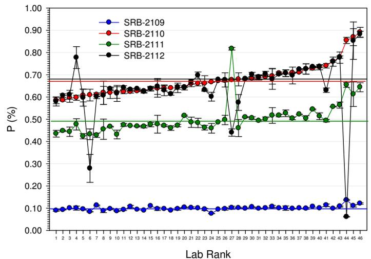
Figure 8. Phosphorus distribution lab plot for SRB materials, ALP 2021 Cycle 46.
