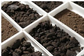
SRS material homogeneity was evaluated based on soil test codes pH (1:1) H<sub>2</sub>O, buffer pH Adams Evans, EC (1:1), P Olsen, K Olsen, NO<sub>3</sub>-N and SOM-WB on analysis of five jars of each PT soil, each in analyzed in triplicate by an independent laboratory. Homogeneity results were within acceptable limits for all soils, with the lowest noted for pH H<sub>2</sub>O. Homogeneity was also evaluated on SRB and SRW matrix sam-
