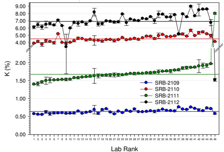
Figure 9. Potassium lab plot for SRB materials, ALP 2021 Cycle 46.
