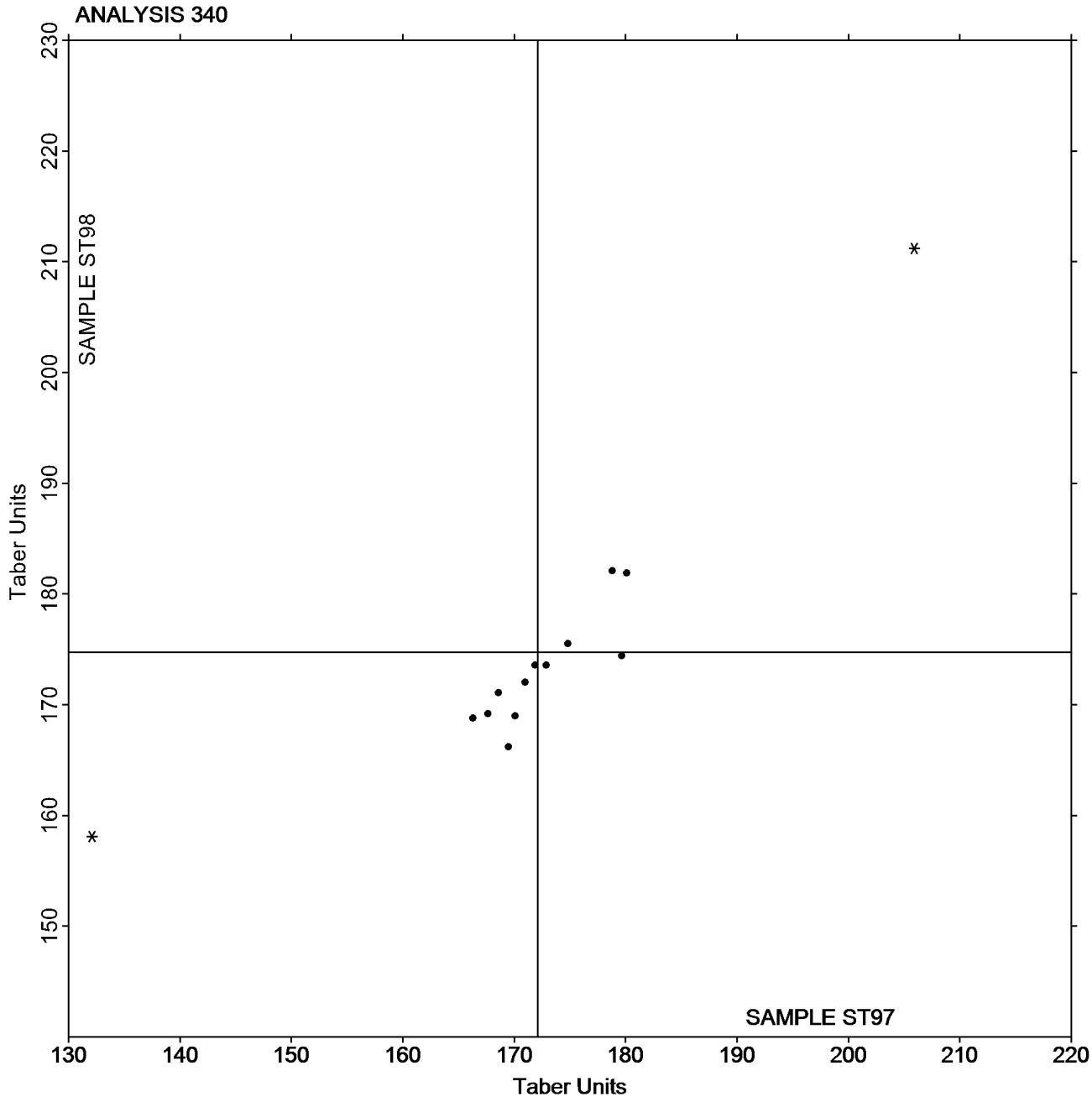
If fewer than 20 laboratories are included in an analysis, a control ellipse will not be drawn on the two-sample plot.
